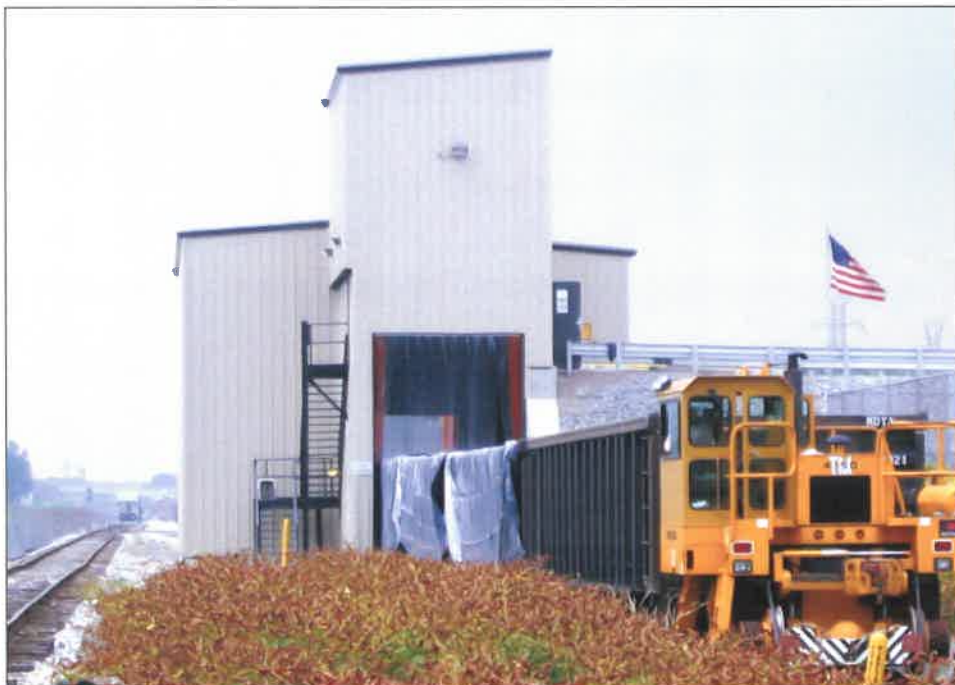
^ Track mobile positioning system lines gondola railcars into North Bergen, NJ transload facility.
